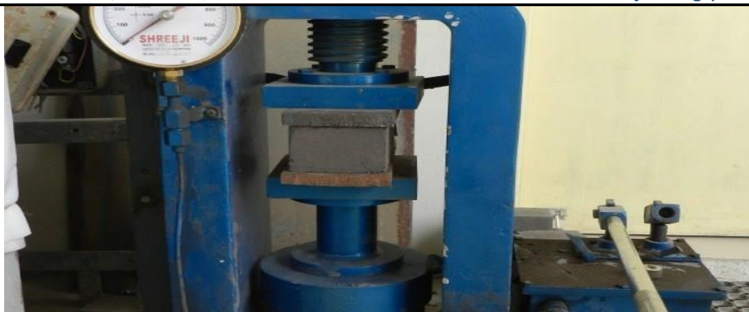
Fig. 3 Compressive strength test
