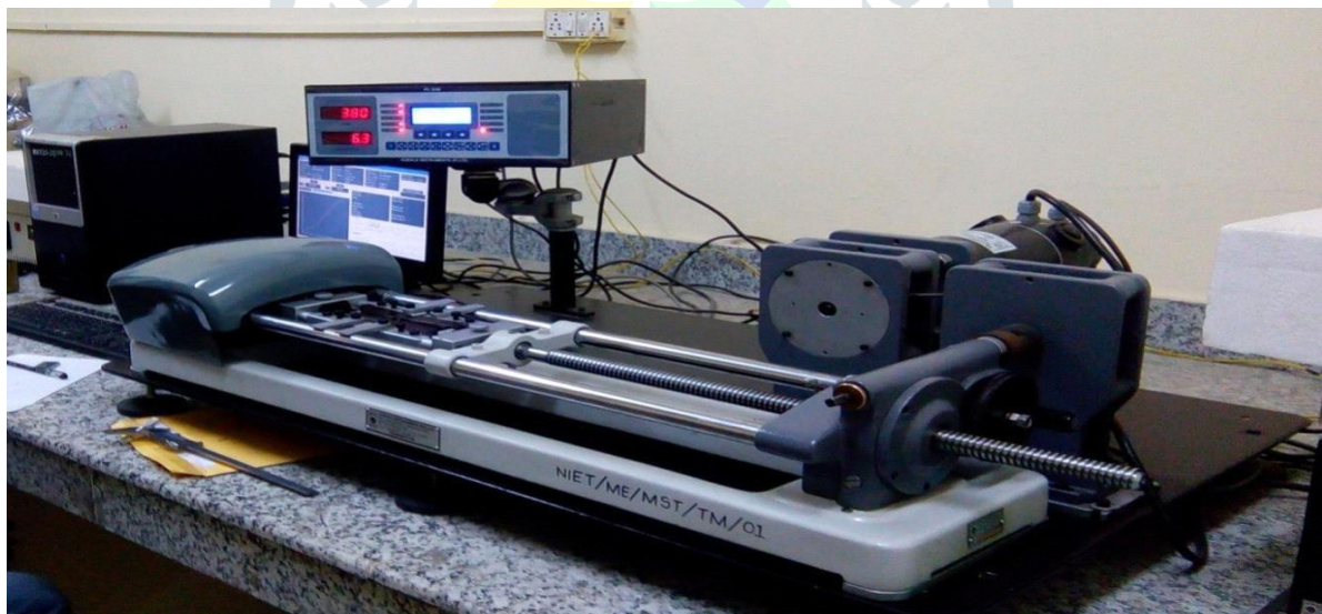
Fig. 4.2. Tensile Testing on Tensometer
