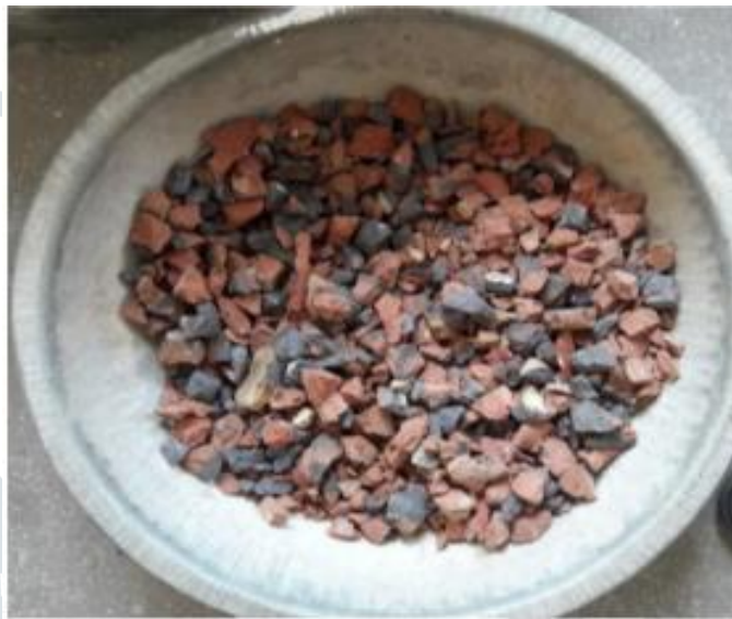
Fig 1- sample of over burn brick aggregate
