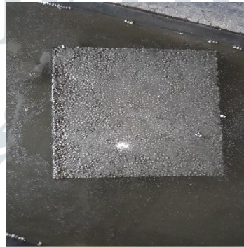
Fig 8.3 Slab floats on water
