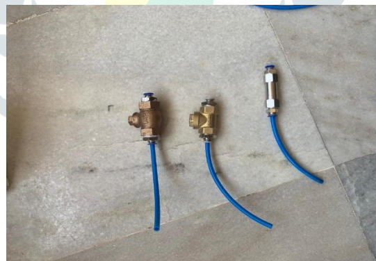
Figure 4.7 Actual image of No-Return Valve
