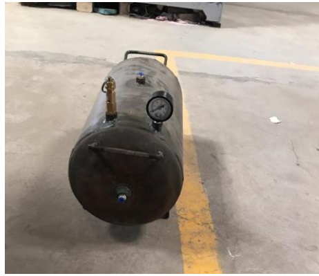
Figure 4.8 Actual image of Surge tank
