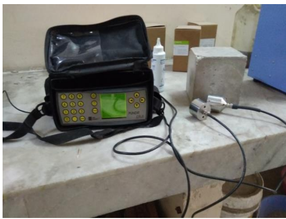
Fig. shows UPV Test apparatus and concrete specimen
