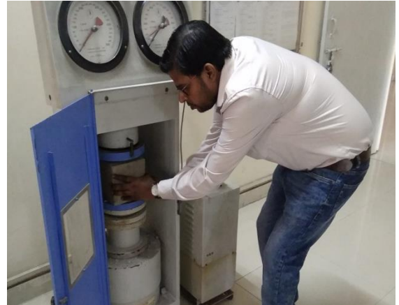
Fig. shows testing of concrete specimen at laboratory
