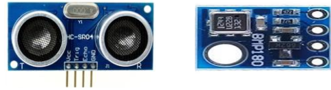
Fig.7 . Ultrasonic and pressure sensor
