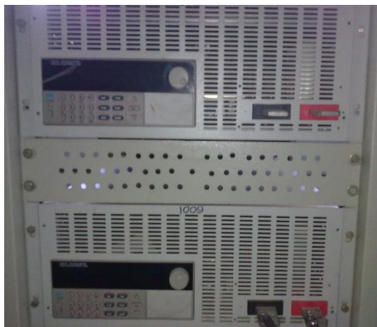
Figure 1 : Image of electronic load bank for discharging a cell.
