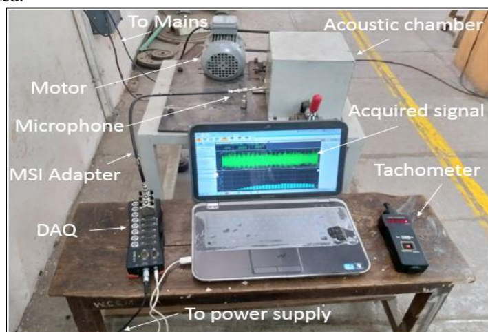
Fig-3: Measuring equipments interfaced with DAQ
