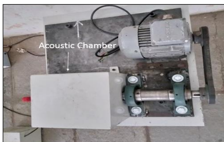
Fig-2: Position of acoustic chamber
