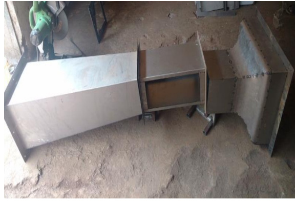
Fig 13: Airflow tunnel during manufacturing
