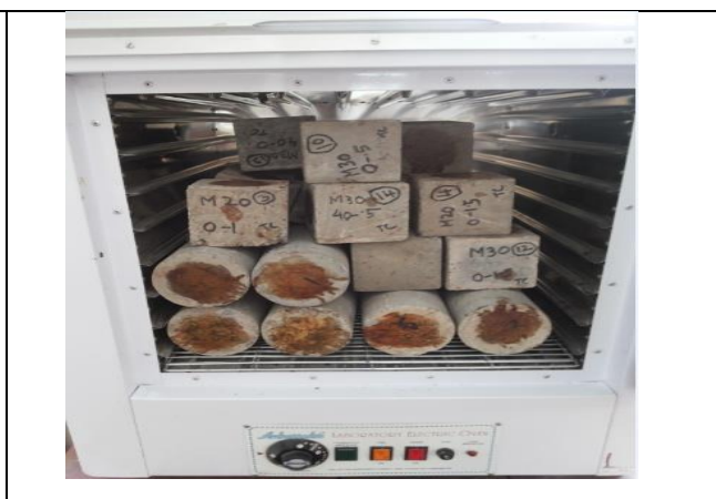
Figure 5: Concrete Specimens Subjected to Elevated Temperature
