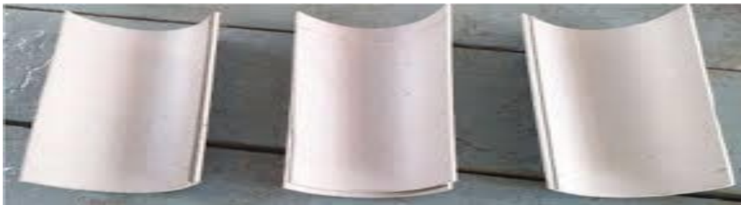
Fig 2.1. Fabricated blades from PVC pipes
