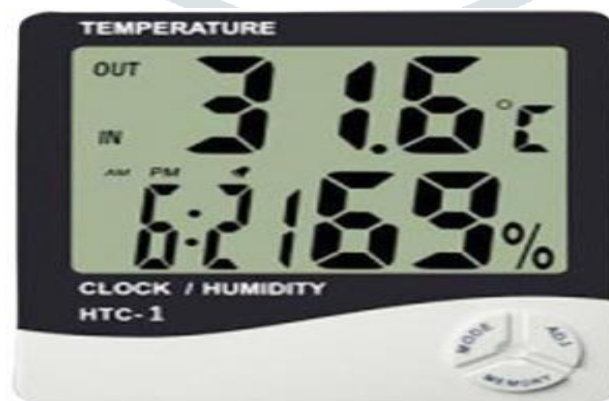
Fig. 6 Hygrometer:- for Measuring of relative humidity in %
