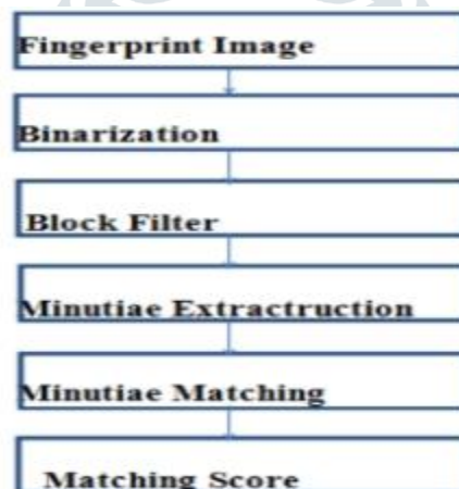
Figure 3 : Flow for Fingerprint Recognition
