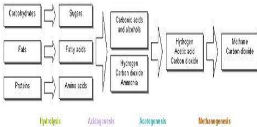
**Figure-1 Stages of anaerobic digestion**
