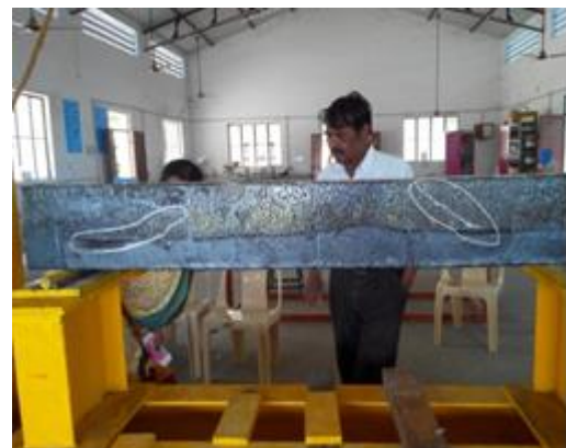
Fig 11 crack pattern on CF-1L Beam
