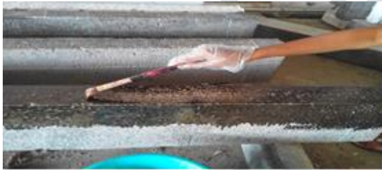
Fig 3: Application of epoxy resin and hardener
