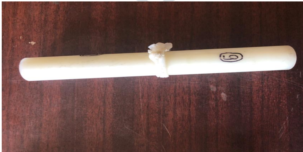
Fig 2 Friction welded joints of Nylon rounds
