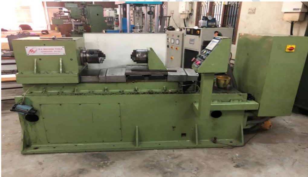
Fig 1 HMT model - Friction welding machine
