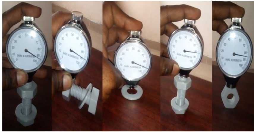
Fig 5 Hardness measurement of bolt and nut assembly
