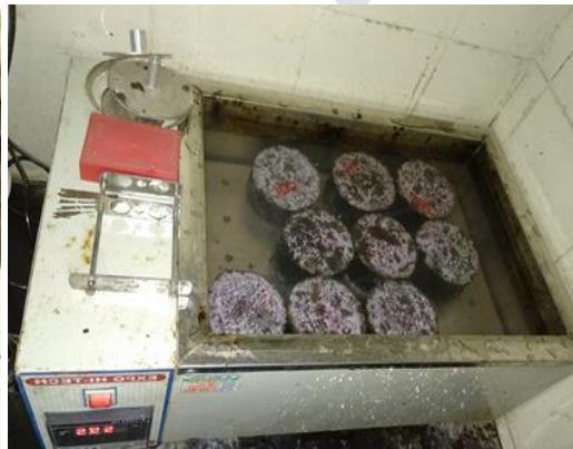
Image 5. CRMB Specimen in Water Bath
