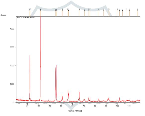
Figure 3 X-ray diffraction of KNbO<sub>3</sub> sample.
