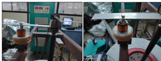
Fig. 3.1 Photographs of the harvesting beam connected to exciter
