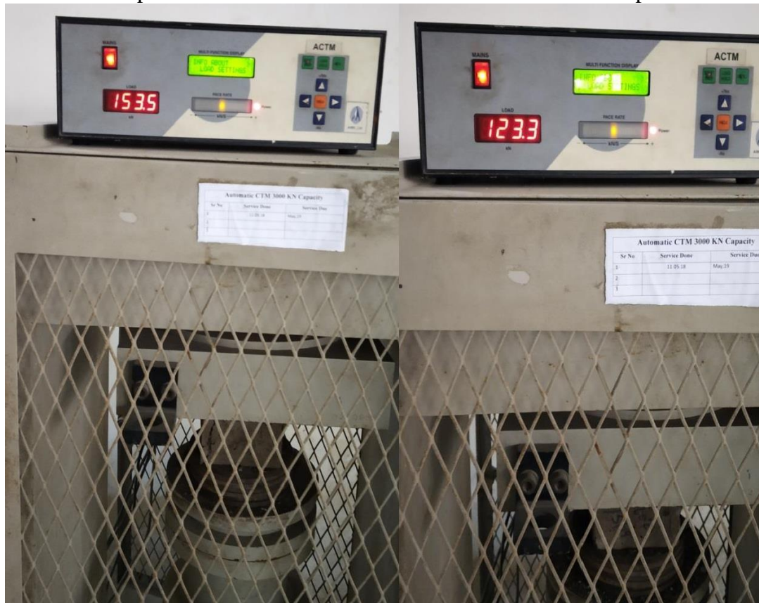
Figure 2 Strength obtain after 7 days of air curing (left image) and Strength obtain after 7 days of water curing ( right image)
