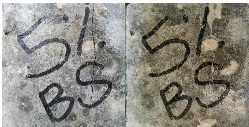
Fig: 2 Bacterial set before and after healing
