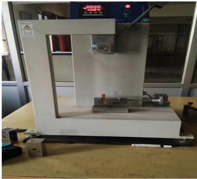
Fig. 2.1.2 Impact testing machine with Sample loaded condition
