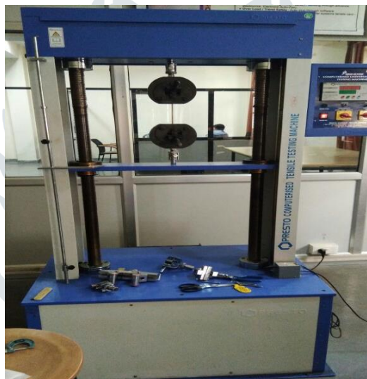
Fig. 2.1.1 UTM machine with Sample loaded condition for tensile testing
