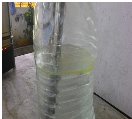
Fig 5.0 The Layer of oil Collected Over the water
