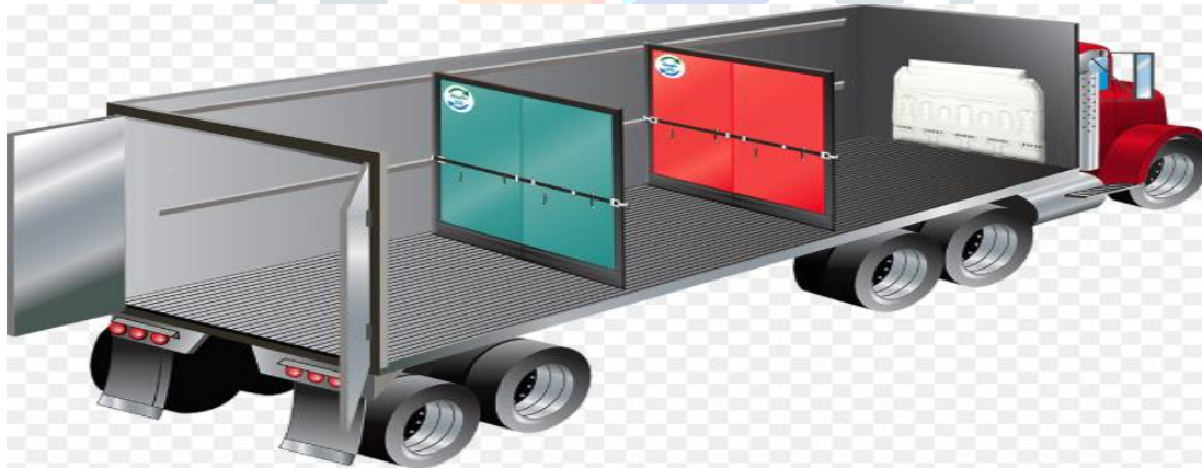
Fig 1: Layout of Transport Refrigeration System
