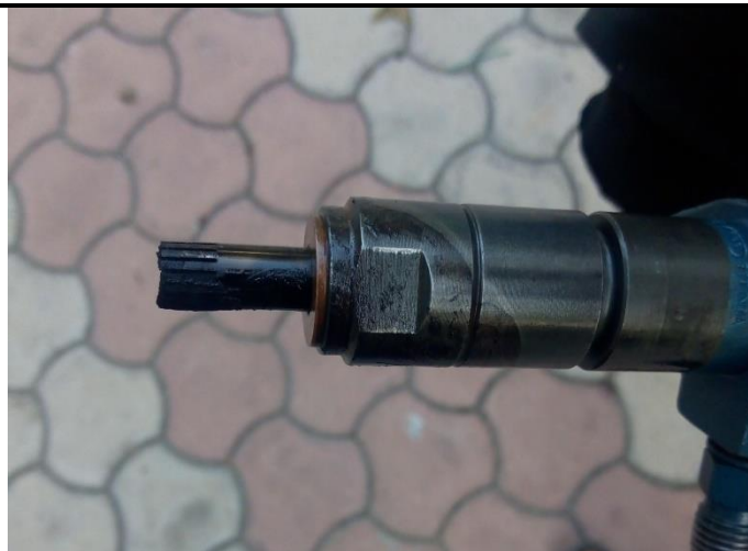
Fig: Carbon deposits on Retrofit after the performance tests
