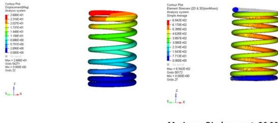
Maximum Displacement- 26.06mm Maximum Stress -694.2 mpa
