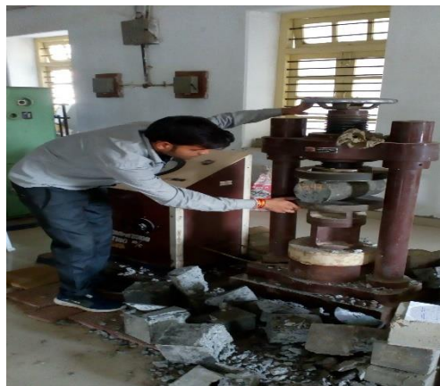
Figure 9. Testing of cylinder specimen
