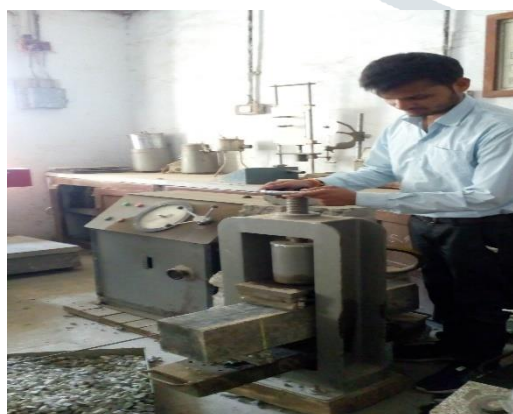
Figure 11. Testing of beam specimen
