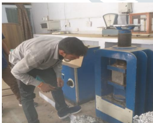
Figure 7. testing of cube specimen
