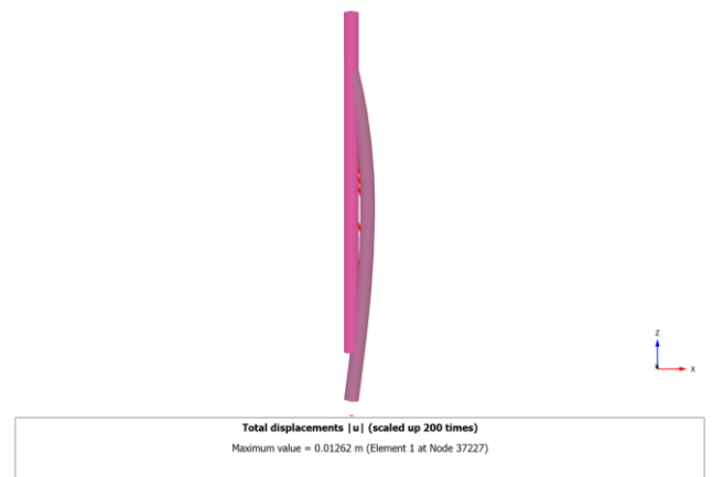
Figure Maximum total displacement of pile with tunnel=12.37 mm
