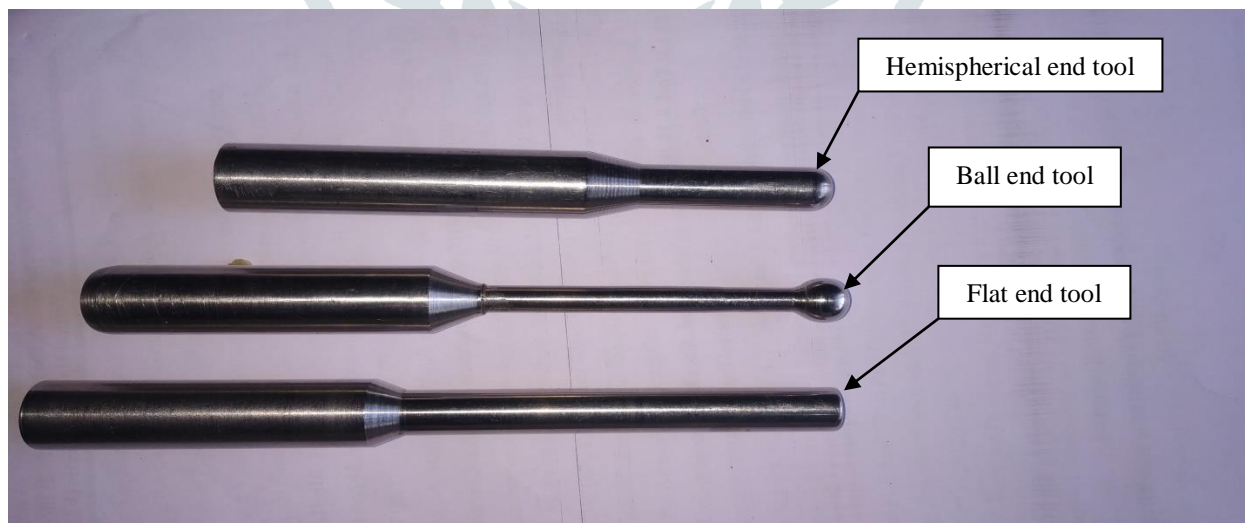
fig. 3: tools with three different profiles
