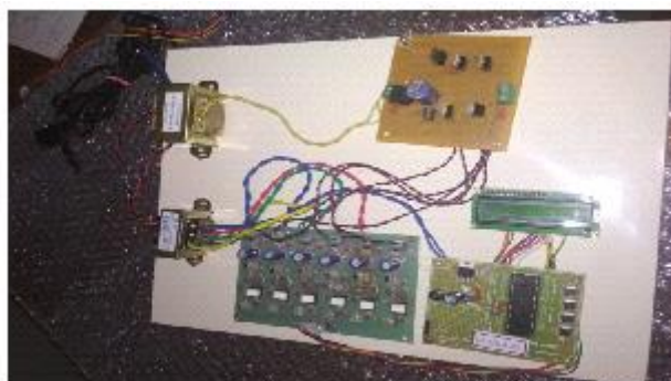
Fig.10. The complete hardware set up for the motor control
