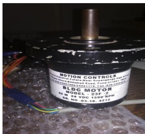
Fig 5. 24 V, 80 W, 1500 rpm BLDC motor
