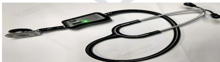
Fig. (1).Ayu lynk attached to normal stethoscope
