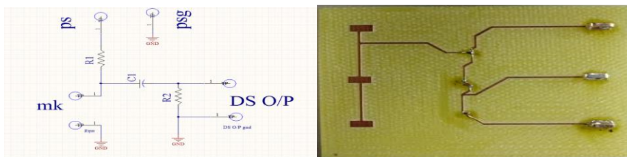
Fig.(6). MIC PCB for acoustic test
