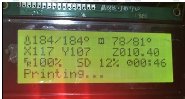
Fig 4. LCD screen displaying the details while 3D printing
