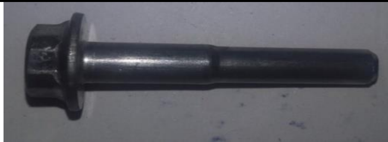
Fig.4 Defects of across Corner Under fill
