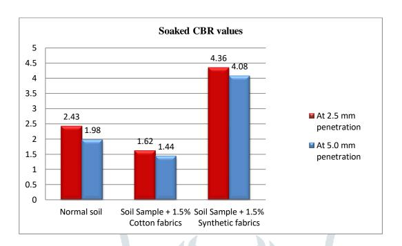
4) Comparison between Normal soil, 2 % Cotton Fabrics mix in soil and 2 % Synthetic Fabrics mix in soil for SOAKED CBR:-
