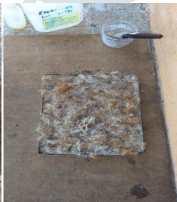
fig b. hand layup technique
