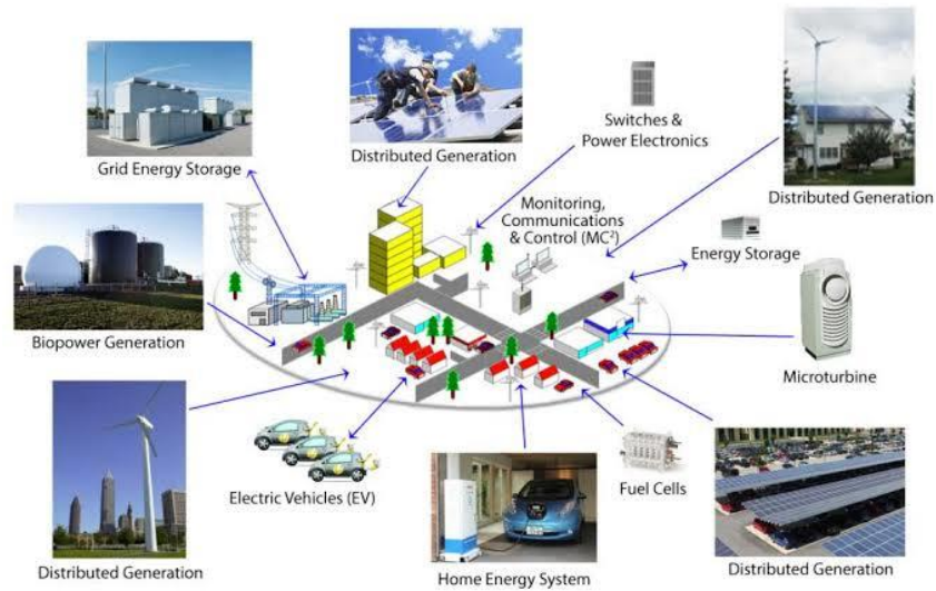
Fig1. Microgrid power system
