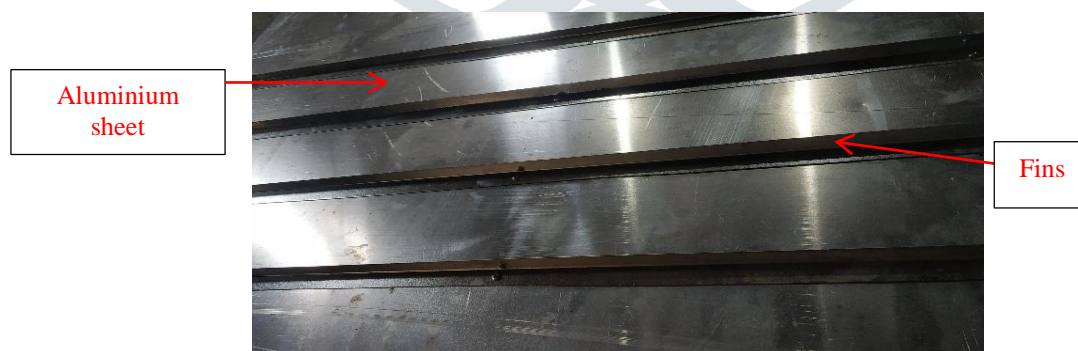
Fig. 3 Internal structure of PCM container
