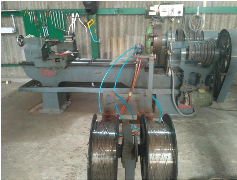
Figure 6.1 : Layout of Two wire electric arc spraying
