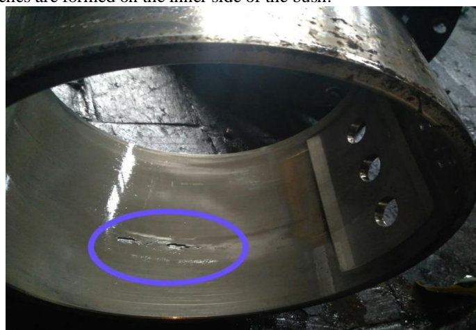
Figure 3.2: Scratches on inner side of the bush
