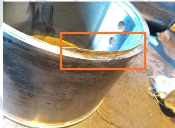
Figure 3.1 : wear out of the babbitt material
