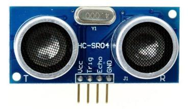
The ultrasonic sensor emits high frequency sound waves through the air and receives the waves reflected from the target. Ultrasonic sensor measures the distance by evaluating the time between emission and reception using the formula:
