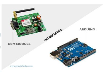
A **GSM Module** is used to send and receive messages. We use SIM800 GSM Module, means the module supports communication in 800MHz band.
