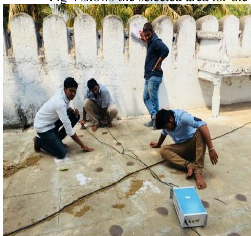
Fig 6 Measuring UPV values on the slab of heritage structure Fig 7 showing bottom portion of the slab
