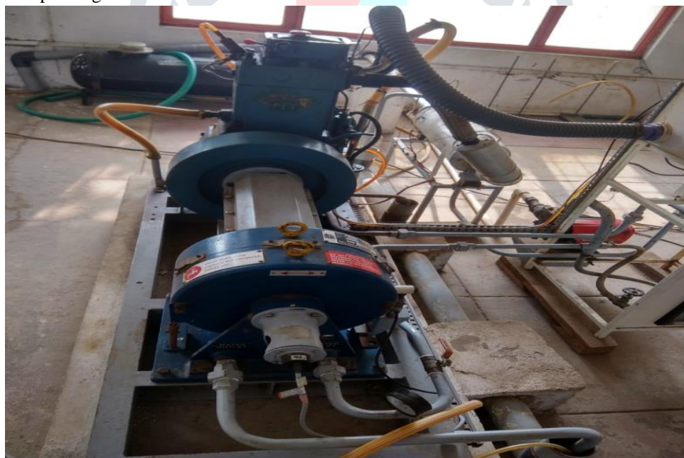
Fig.1 4-Stroke Diesel Engine with eddy dynamo meter
