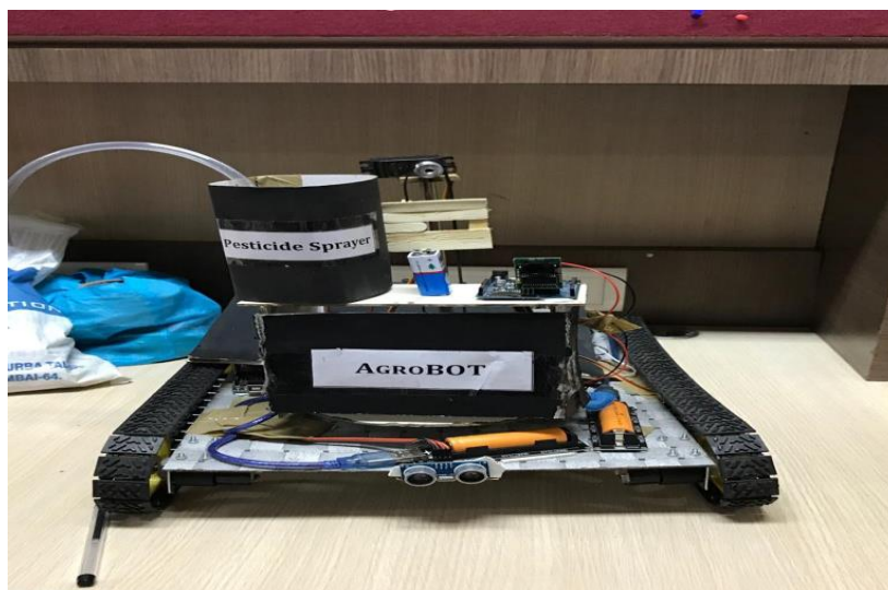
Figure 5: Agrobot with Pesticide Sprayer.
