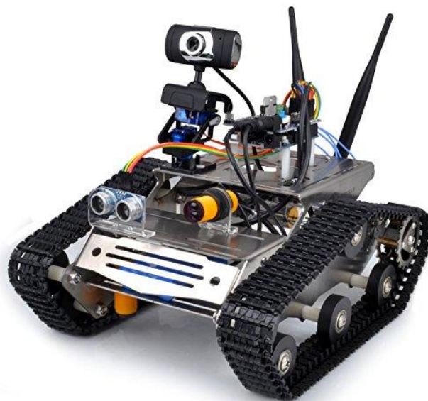
Figure 1: Wireless Robot for Capturing Live Images of crops
