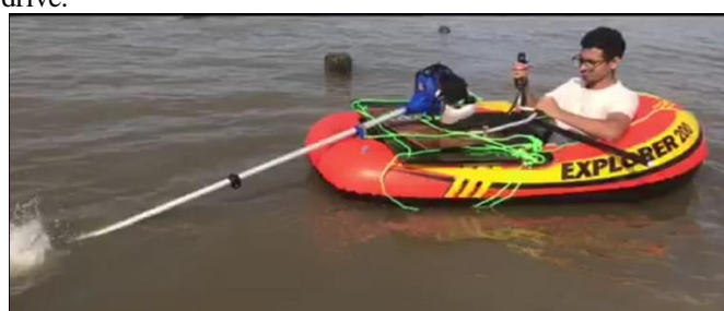
Fig 5.1: Testing of the engine with boat on gorai beach
