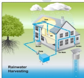
Fig.2 the rooftop harvesting
