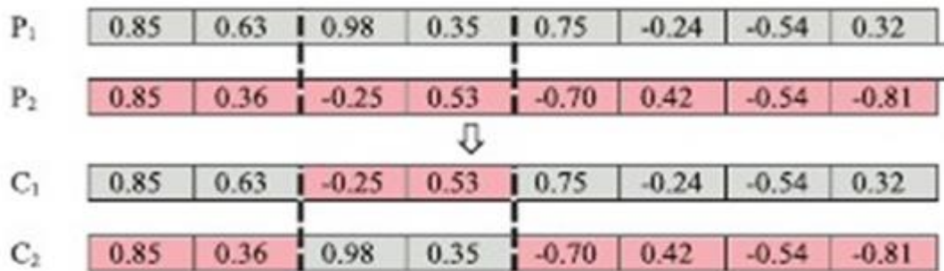
Fig. 2. Two-point crossover. P1 and P2 are the selected parents while C1 and C2 are the generated children.
