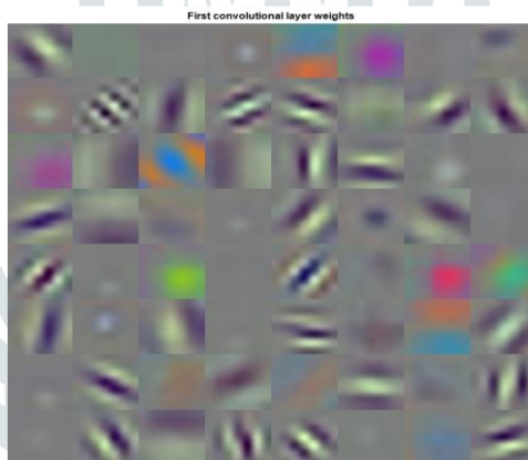
Fig 7. The visualization of the learned First convolutional layer features in the trained CNN.
