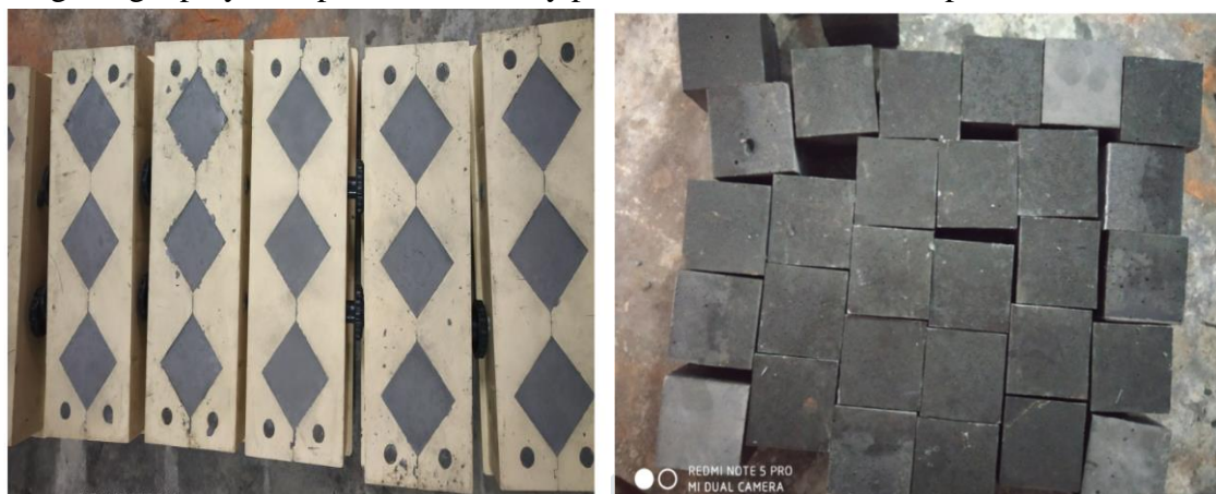
Figure 3. Geopolymer Specimen prepared using 50*50*50 mm plastic moulds
