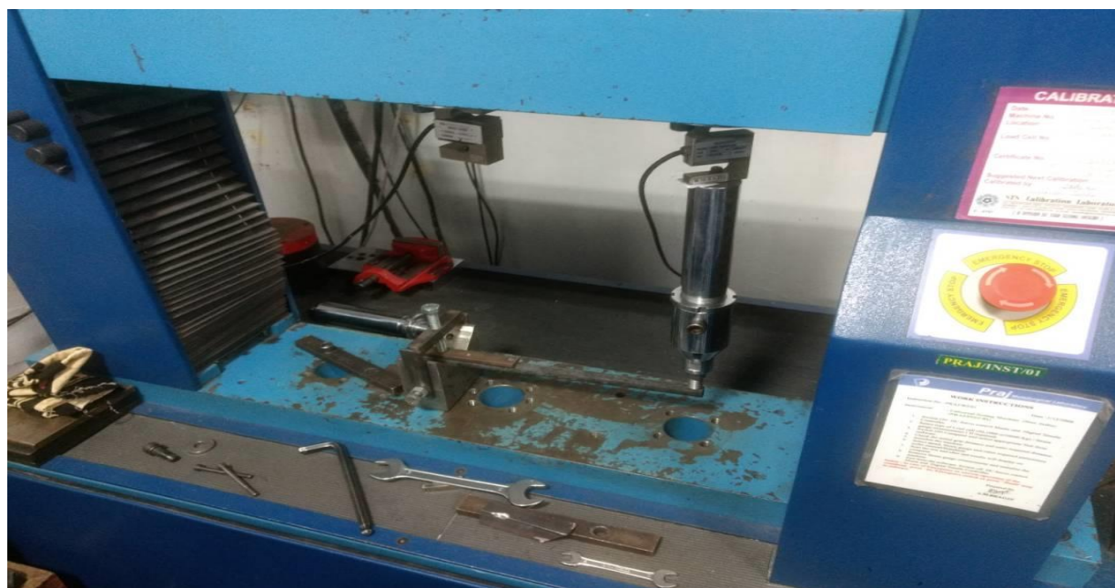
Fig.15 Testing of Shaft on UTM
